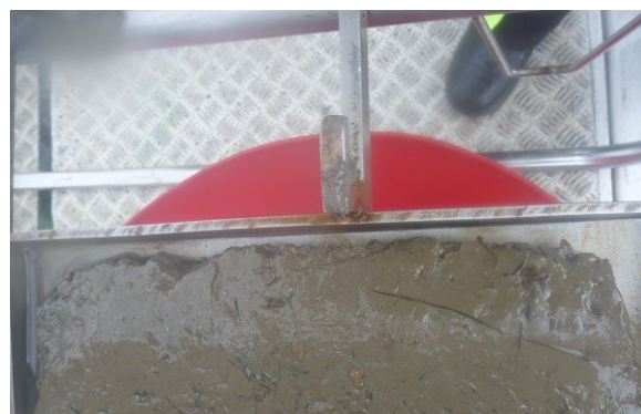
Soft mud sample in Day Grab before taking sub-samples for lab analysis.
